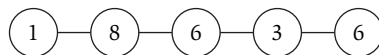
Figure 6.28 A paths with weights on the nodes. The maximum weight of an independent set is 14.
